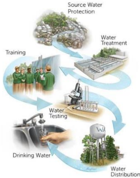
Municipal System - Multi barrier approach to protecting drinking water
