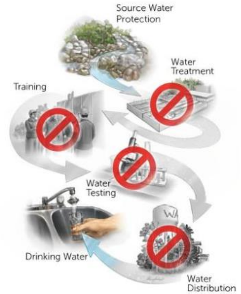
Private System - No multi-barrier approach to protecting drinking water
